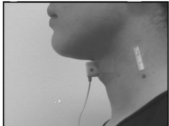
Fig.3 Displacement measurement of throat surface
