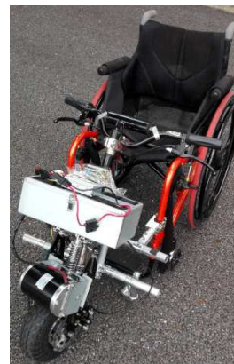
Fig.7 Wheelchair equipped with a removable drive system installed
