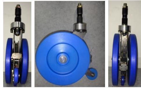
Fig. 10 Prototype of step-climbing casters
