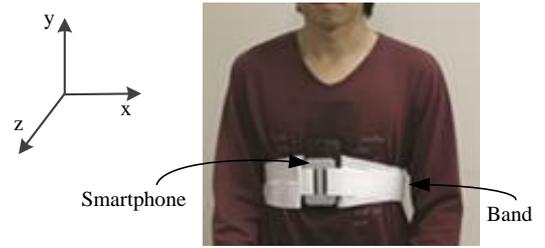
Fig. 2 Android smartphone being strapped on the user chest
