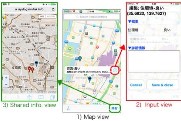
Fig.2 User interface of smartphone application for sharing accessibility conditions
