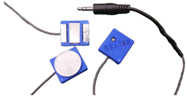
Fig. 3 Small dry-electrode EMG sensor
