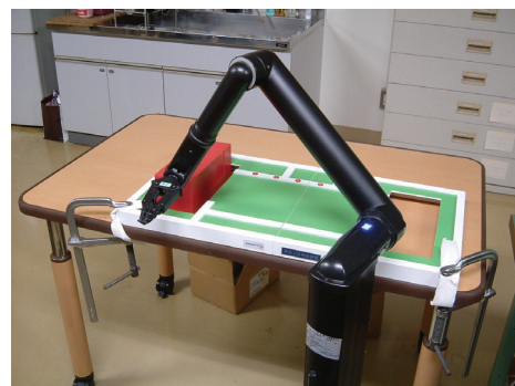
Fig. 1 Assistive robotic arm (iARM, Exact Dynamics) and STEF (SAKAI Medical Co., Ltd.)
