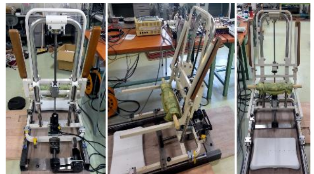
Fig. 2 Experiment device for sit-to-stand analysis
