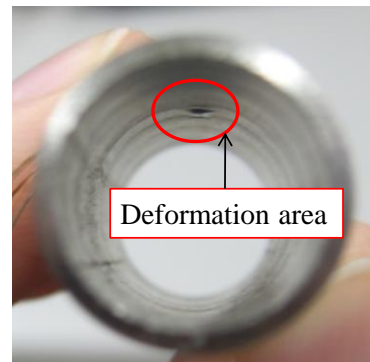
Fig.7 Deformation area in the test model having a wall thickness of 0.01 mm
