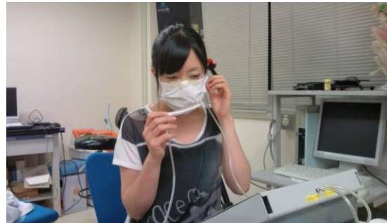
Fig. 5 Measurement of leakage rate using Mask Fitting Tester
