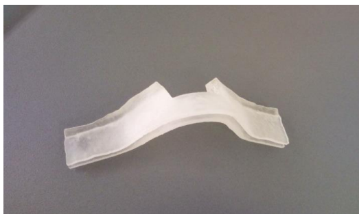
Fig.4 Mask-fitting piece fabricated using 3-d printer
