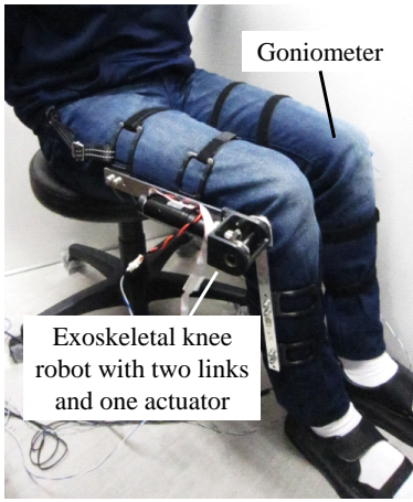
Fig.1: Exoskeletal knee robot worn by healthy human (right leg). Goniometer (left leg, hidden).
