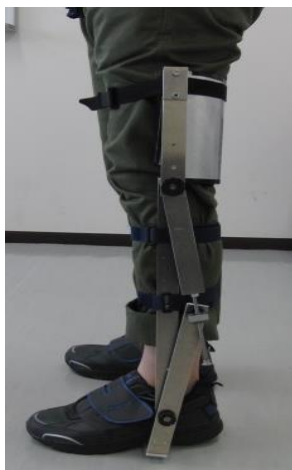
Fig.5 Developed knee orthosis
