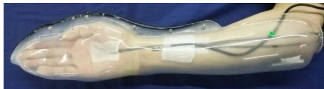
Fig.1 Quasi-transradial prosthetic socket with sensor installed
