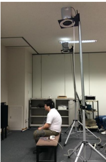
Fig. 3 The measurement setup for the experiment 2. The subject was presented the sound from ceiling speakers.
