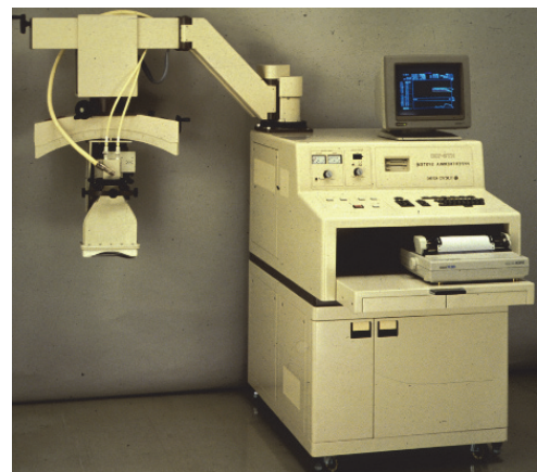
Fig. 7 Photo of heating system using lens applicator.
