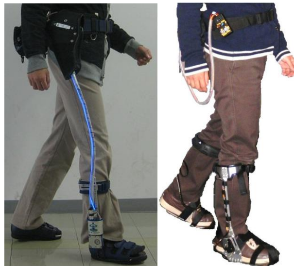
Fig. 1 Comparison between the flexible shaft and worm gear type (left photo) and the servo motor type (right photo) of the assistance apparatuses
