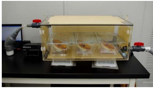
Fig.5 Chamber for filling bad odors
