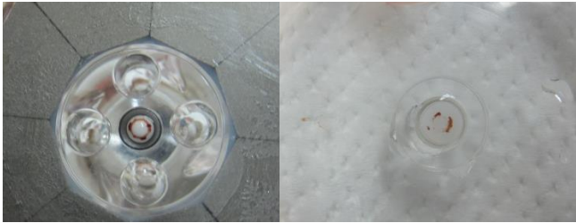
Fig. 8 Thrombus surrounding pivot bearing
