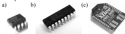
Fig.5 ICs in the electric circuit a) Instrumentation amplifier, b) dsPIC microcontroller, and c) wireless communication module
