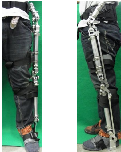
Fig.2 Power Assist Suit adapted to bi-articular muscles model
