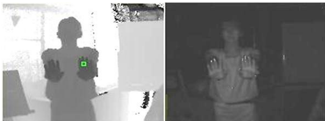
Fig.2 The picture outputted from a ToF camera
