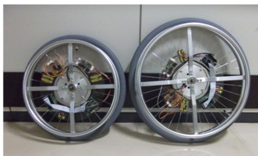
Fig. 2 Appearance of measuring system for assessment of wheelchair driving capability(left:20-inch wheel, right:24-inch wheel).
