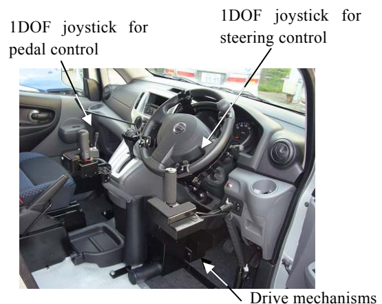
Fig.1 The developed joystick system installed on a van
