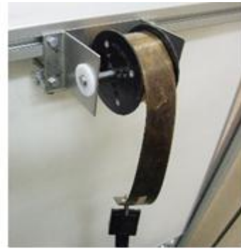
Fig.4 Device to Unload Patient's Weight
