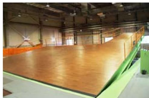
Fig2. Test equipments of stability test on inclined surface
