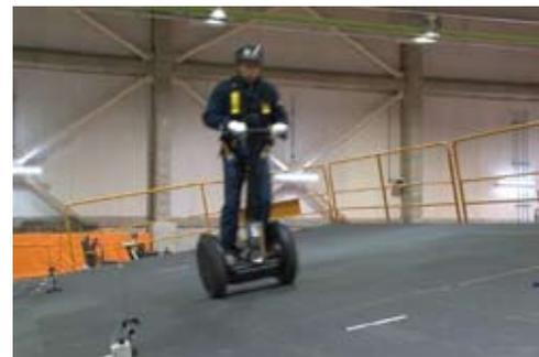
Fig6. An example of stability test during traveling on a laterally inclined surface
