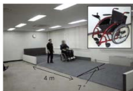
Fig. 1 Test course with a 7-degree cross slope. A test wheelchair with the DTPC is shown in the inset.
