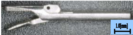
Fig. 3 Micro Grasping forceps (1mm in diameter)
