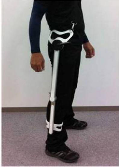
Fig.3 Walking-assist device (mono type)
