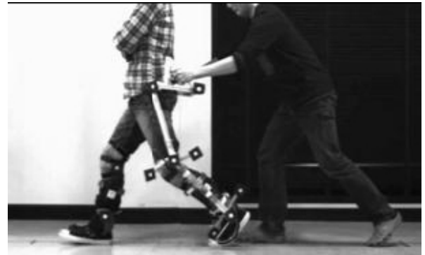
Fig.2 Walking-assist device (biped type)
