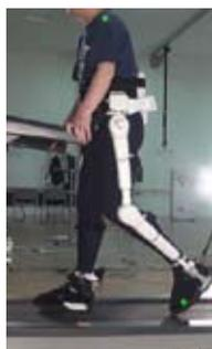
Fig. 1 Robot Suit HAL (Hybrid Assistive Limb)
