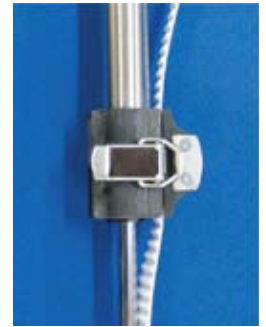
Fig. 11 Timing belt-length adjusting mechanism
