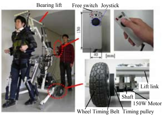
Fig. 3 Photos of the apparatus and weight bearing lift
