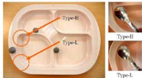
Fig. 2 Two different edges of Melamine partition plate TM tested: Type-H is conformed to the tip of Light spoon TM , while Type-L is not conformed to that.
