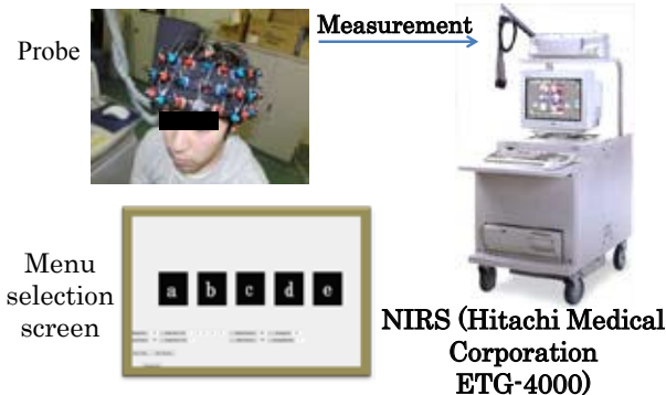
Fig.1 Configuration of the measuring system using NIRS
