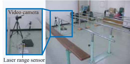
Fig. 7 Experimental setup for leg position measurement
