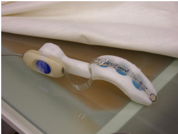
Fig. 1 RAPUDA finger with force sensor
