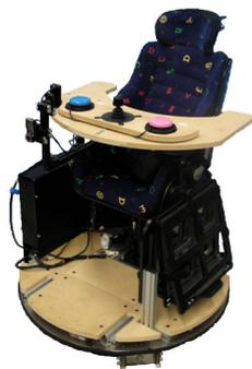
Fig.1 Prototype of mobile support equipment (Omni-directional movement type)
