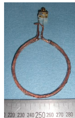
Fig.12 Measurement device of blood relative permeability using coaxial cable coil of 2 turns
