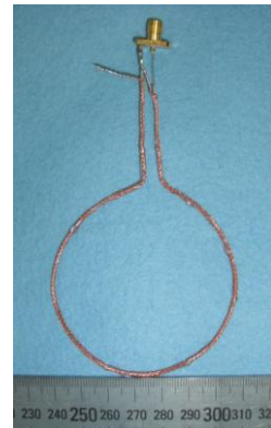
Fig.6 Measurement device of blood relative permeability using coaxial cable coil of 1 turn
