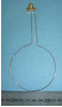
Fig.8 Measurement device of blood relative permeability using a solid wire
